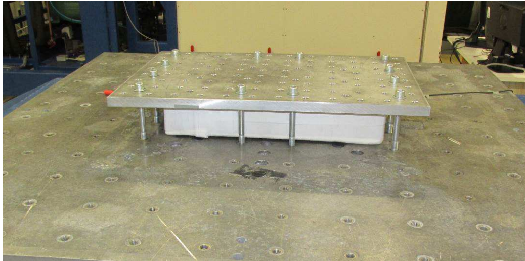
Picture 6 test setup for T.4 – mechanical shock test, z-axis
