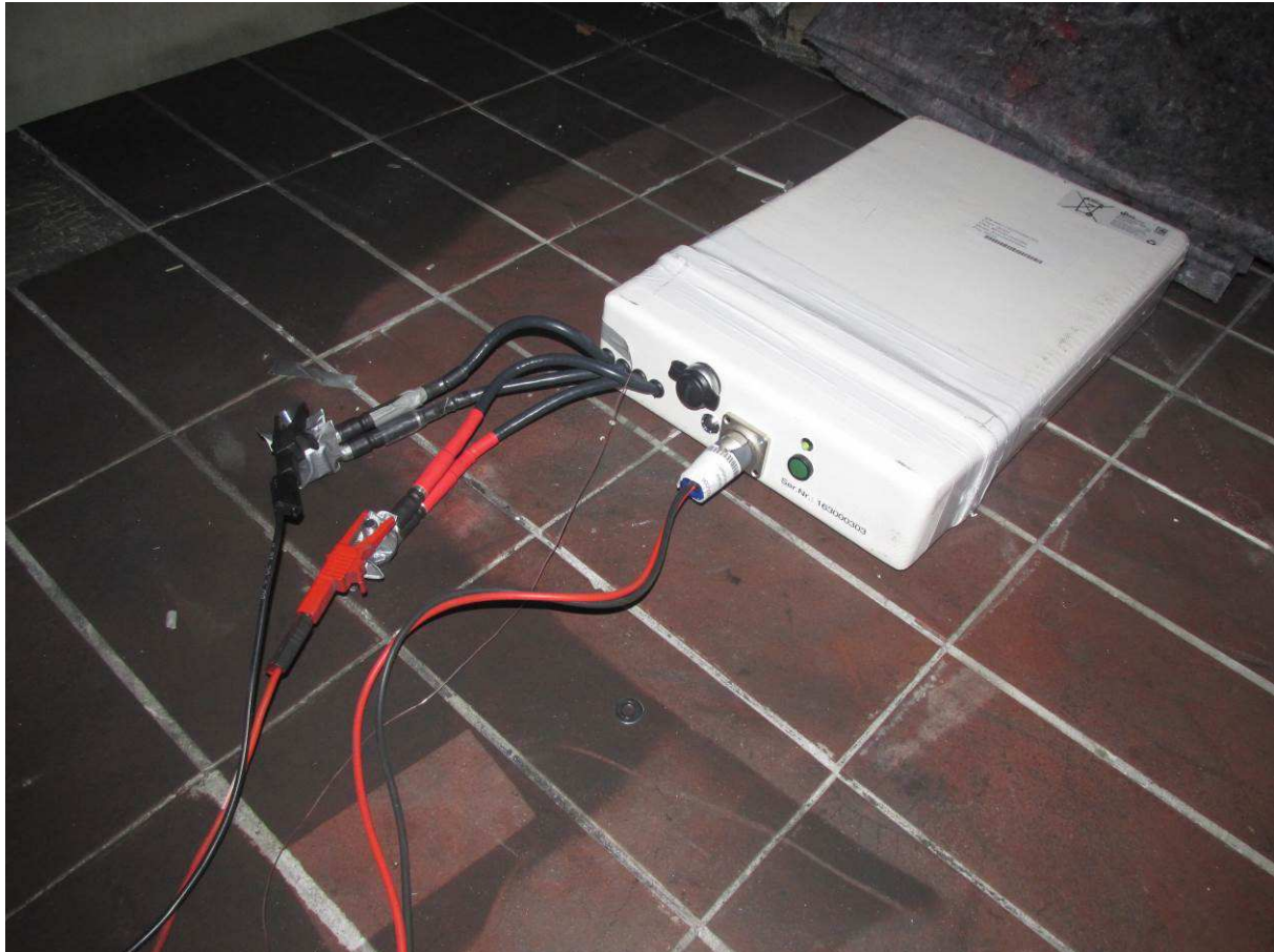
Picture 10 test setup for T.7 - overcharge test
